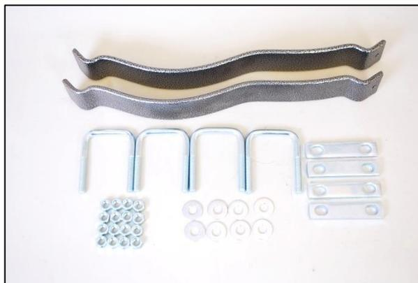
Factory leaf springs are not designed with performance and acceleration in mind. Under acceleration (and even extreme deceleration) the rear end housing wants to rotate and can cause the leaf springs to wrap or twist resulting in wheel spin and driveline damaging hop.
