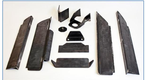
The new Frame FX kit is made up 14 pre-cut 10-gauge steel panels that match the thickness of the factory frame and fit into the weak points of the factory chassis. Hellwig also engineered another panel that adds an extra mount to tie the floor to the chassis to add even more strength to the entire car. In addition, brackets are provided to mount the transmission crossmember with enough adjustment to accommodate nearly any drivetrain configuration.
