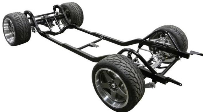
The front suspension features upper A-arms fit with needle-bearings that are engineered with separate camber and caster adjustments (without using shims). In the rear you'll find a four-bar system with teflon-lined spherical rod-ends for bind-free operation and a smooth ride. The Schwarz chassis incorporates longer shocks at all four corners than any other chassis to improve the overall handling and tuning of the suspension.
